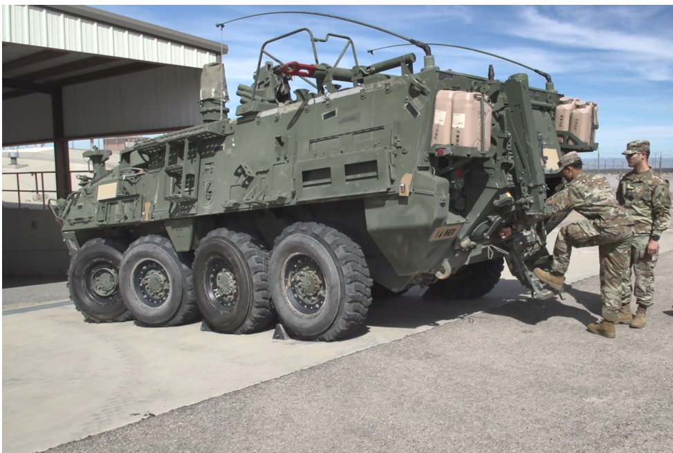
Figure 2. Soldiers from the 1st AD 16th BEB recover radiation detection equipment between test shots from the Stryker NBCRV at the White Sands Missile Range Fast Burst Reactor.
