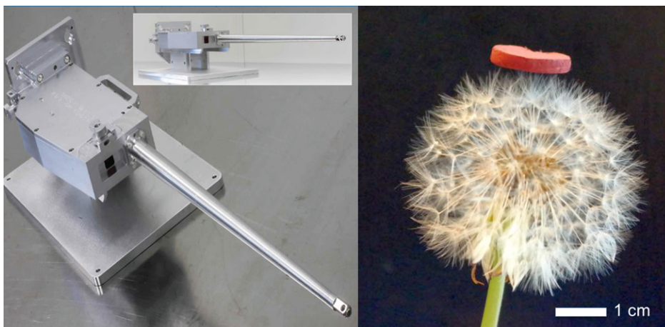
Figure 4. National Ignition Facility X-ray Spectrometer (left) and ultra-light copper foam x-ray targets (right).
